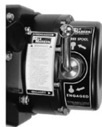
3-1: Clutch Engagement: SEC/PEC Models
