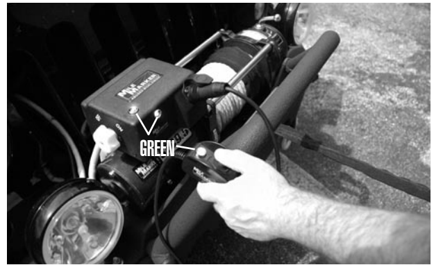
3-8: Toggle Down: Power in, "Green" LED
