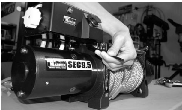
2-4: Secure Box With Allen Wrench
