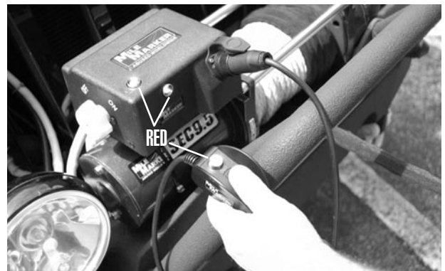
3-9: Toggle Down: Power out "Red" LED (FOR INTERMITTENT USE ONLY)
