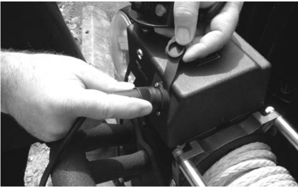
3-4: Tighten Thread Lock
