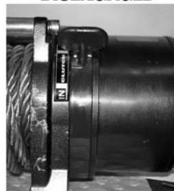
3-2: Clutch Engagement: PE/E Models
